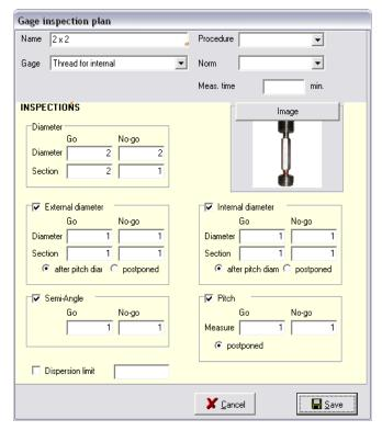
Detailed inspection plans can be created for solid gages and instruments.
