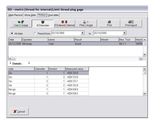
It is possible to browse through all measurements done in the past as well as check the list of data acquired during each measurement section.
