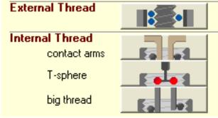
Wire and ball measurements are support with automatic selection of the best measuring tool (wire or ball) to be used for the measurement.
