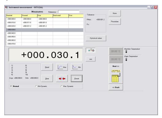
The software **guides the operator** through the measurement procedures and calculates the instrument limits in terms of maximum deviation, error at each step, hysterisis, repeatability and reproducibility of the measures.
