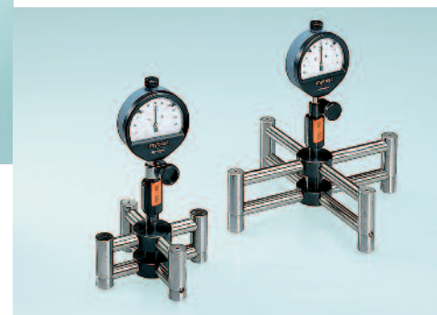
Cross sleeve with runners for dia. 130-800 mm for deep bores or through bores, alignment in the bore is made through the 4 runners
